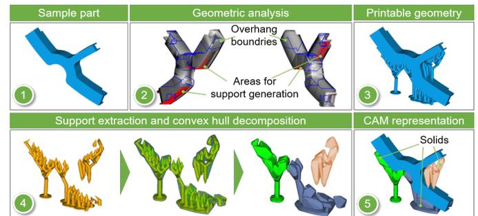
Fig. 3. Solid (BREP) generation using a hierarchical convex hull decomposition
