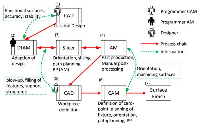
Fig. 1. Sample process chain of hybrid AM today
