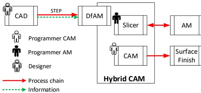
Fig. 2. Hybrid process chain with hybrid CAM
